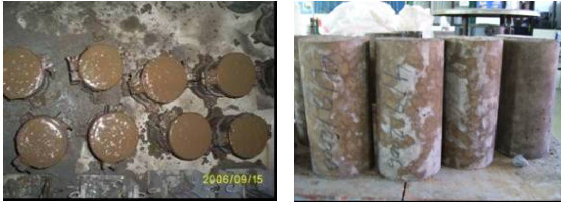
Figure 4. (a) Geopolymer Concrete Mixture in the Steel Moulds (b) Concrete Specimens
